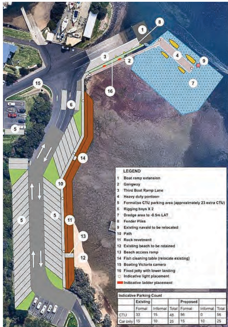
Under this new draft concept plan for an upgrade of the Newhaven boat ramp, there will be a dredge area to create better access for boaters at a range of tides, an extension to the seawall and rock revetment, alongside a third boat ramp lane, ramp extension and pontoon.
