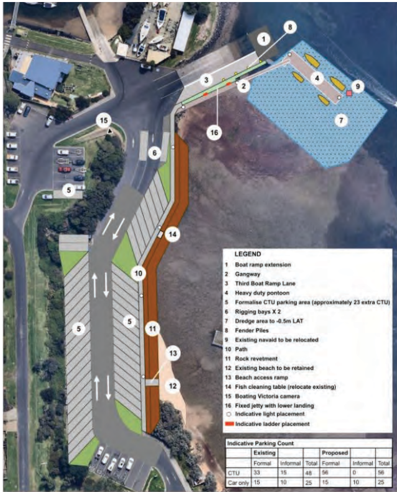
This 2023 draft concept plan for an upgrade of the Newhaven boat ramp, proposed to dredge to create better access for boaters at a range of tides, with works including an extension to the seawall and rock revetment, alongside a third boat ramp lane, ramp extension and pontoon. The plans are yet to be funded.
